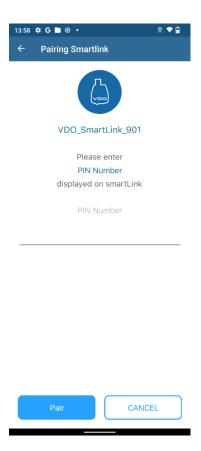
4. The phone will automatically connect to the DTCO and the device will display a token code that you should enter in the app, also
